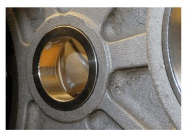
The main casing has been strengthened, by machining the bore of the intermediate shaft allowing a steel bush to be inserted, preventing the aluminium wearing from the head of the intermediate shaft. This is a common fault and ultimately results with leaks. (See image above.)
