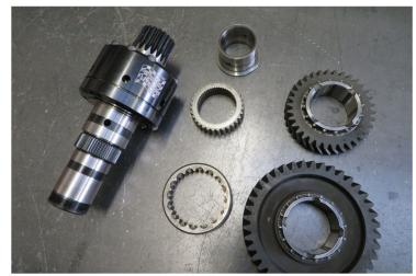
The Stage 1 box uses the original main shaft and diff housing but we fit a billeted heavy duty cross pin replacing the 2 existing pins.
